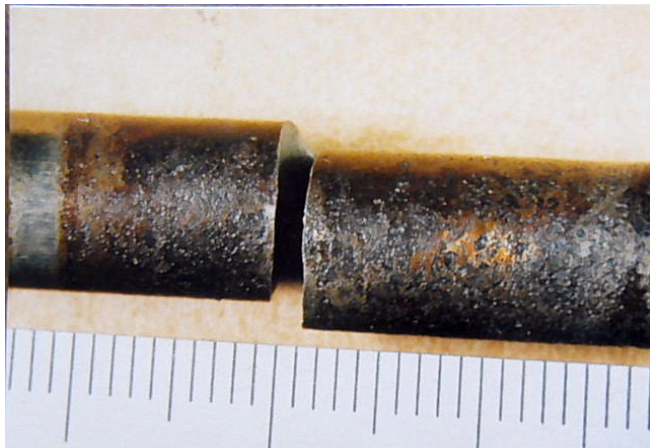
Picture-1 Pitting corrosion of dangerous area
